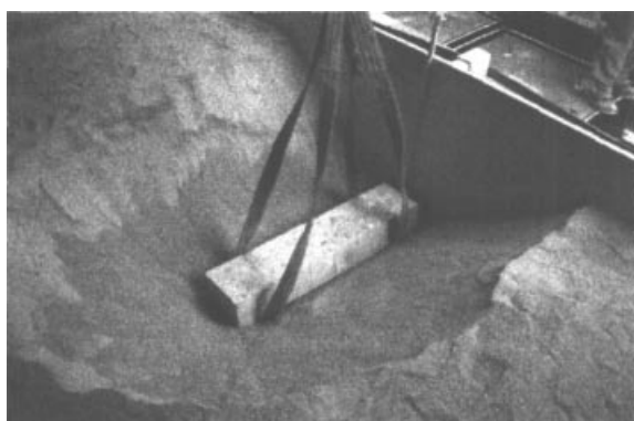
Figure 5. Photograph of sand box during the process of burying the lower wall. Change in grain size at the walls of the ditch due to gravitational separation around the block is clearly visible and could be imaged with GPR (see Figure 4b).
