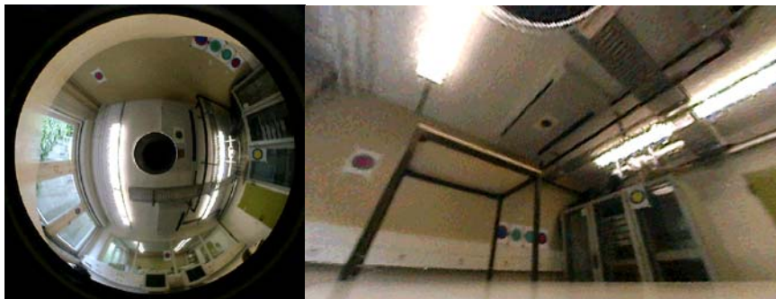
Figure 3: A 360^\circ image and its cartesian reconstruction. The image resolution is 640 \times 480 pixel; this can be seen in the coarse reconstruction results, especially towards the top of the picture.
