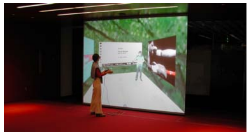
Figure 1: Telepresence in action in the blue-c. The customer sees the remote sales clerk as a 3D representation inside the virtual shop environment.
