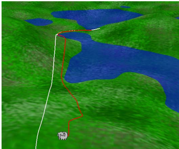
Figure 10: The resulting path (white) and the movement adapted to the slope of the terrain (red).
