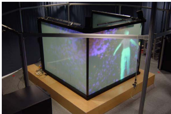
Fig. 8. The blue-c: An immersive telepresence installation allowing simultaneous acquisition and projection.
