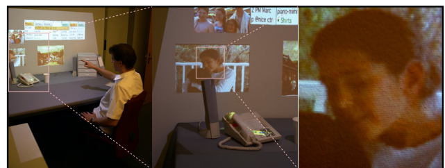
Figure 4: Three different levels of magnification of the projection in operation. Note that the dithering is completely invisible in actual scale, and no visible hint of the embedded binary image can be found.
