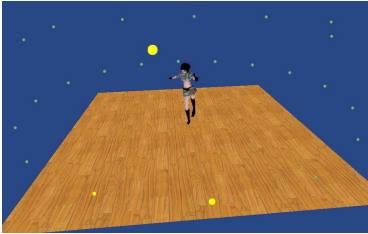
Figure 5: Illustration of view-dependent camera weighting. Green dots indicate the inactive and yellow dots the rendering-active cameras. The size of the circle corresponds to the camera rendering weight for the virtual viewpoint of this rendering.
