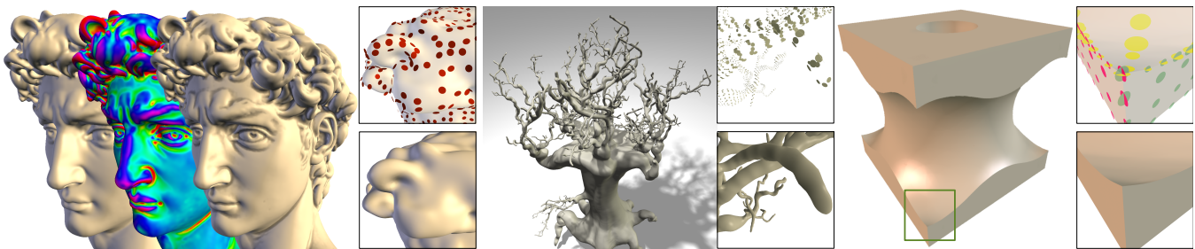
Figure 1: Illustration of the central features of our algebraic MLS framework. From left to right: efficient handling of very complex point sets, fast mean curvature evaluation and shading, significantly increased stability in regions of high curvature, sharp features with controlled sharpness. Sample positions are partly highlighted.
