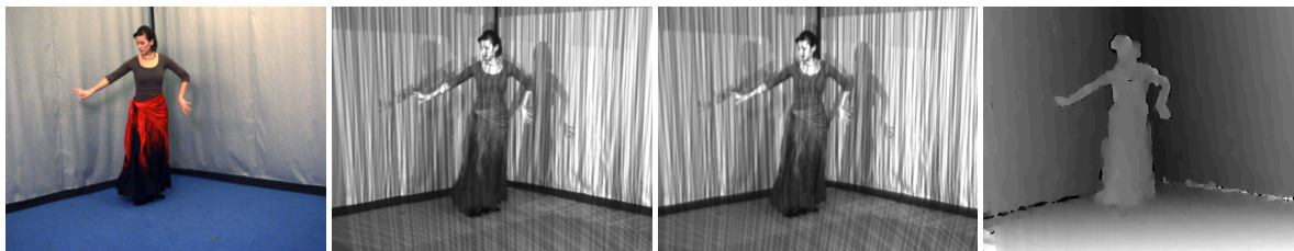
Figure 13: Input color and structured light images of the Flamenco dataset [WWG06], and the resulting disparity map reconstructed by stereo vision on structured light without sub-pixel estimation.
