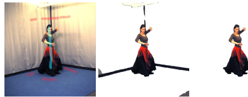
Figure 8: Graph cut segmentation using the input image with user markings on the left. Results of the optimization considering colors only (middle) and additional depths (right).
