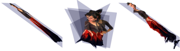
Figure 2: Illustration of the billboard cloud for one object: Billboard plane from one input view (left), composition of planes from multiple input views to a billboard cloud (middle), displacement-mapped billboard plane from one input view (right).
