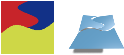
Figure 7: Two complete, intersecting cuts through a single element, resulting in three separate connected components.
