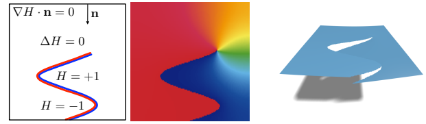
Figure 8: A partial cut in a single element: The corresponding Laplace problem (left), the resulting harmonic enrichment texture (center), and the element behavior in a simulation (right).
