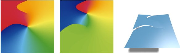
Figure 9: Multiple progressive cuts within an element: The harmonic enrichment textures H^i(\xi) for each of the cuts (left, center), and the resulting simulation behavior (right).
