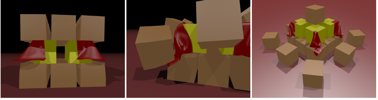
Figure 4: Unified Contact Solver. Our constrained dynamics approach naturally supports diverse deformation models in a unified solver. In the figure, rigid bodies are yellow, linear co-rotational FEM models are orange, and mass-spring cloth is red. The left and middle images show the robust handling of cloth compressed between rigid and deformable solids.
