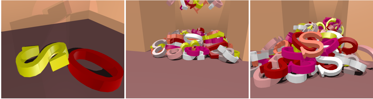
Figure 7: Stacking Deformable Letters. This animation shows accurate geometric handling of sharp features, as well as physically robust impacts, sliding, and stick-slip effects, at large time steps (30 ms).
