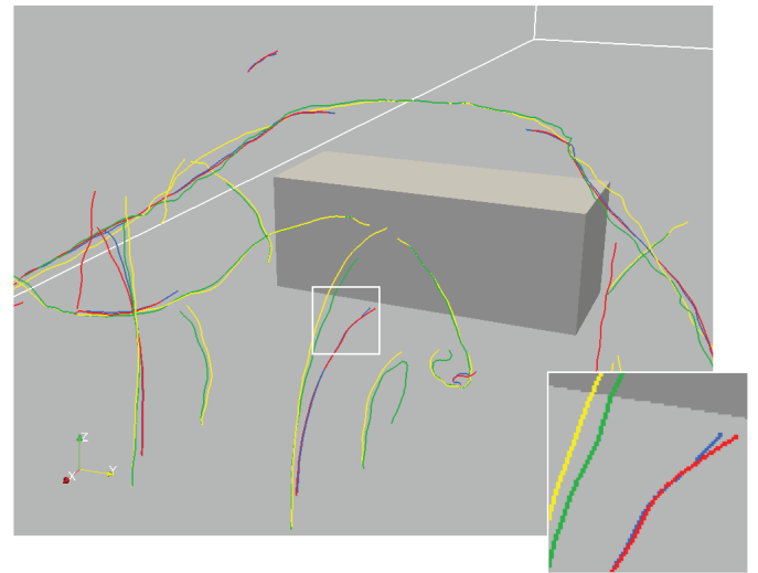
Fig. 6. Comparison of vortex core line criteria, Levy et al. (yellow), Sujudi and Haines (green), Weinkauff et al. (blue), Fuchs et al. (red). Closeup of the vortex analyzed in detail in the accompanying video. The vortex chosen is one of the quasi-symmetric pair of strongest vortices. Results of the methods designed for steady / unsteady flow are pairwise similar.
