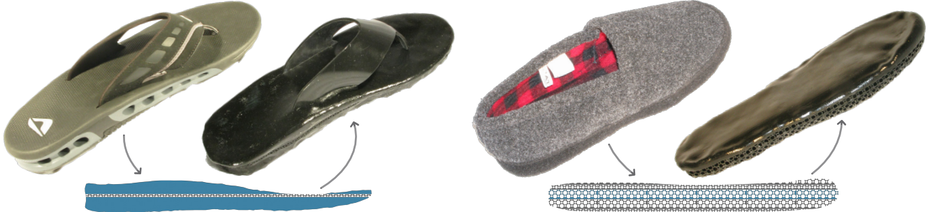
Figure 1: Two examples of real and replicated objects. Thanks to our data-driven process, we are able to measure, simulate, and obtain material combinations of non-linear base materials that match a desired deformation behavior. We can then print those objects with multi-material 3D printers using two materials (blue and black) with varying internal microstructure.
