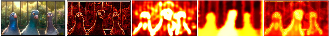
Figure 5: Individual saliency components and final automatically generated saliency map for a scene. From left to right: left image of a stereo pair, local edge saliency, global texture saliency, disparity-based saliency, combined saliency map S .
