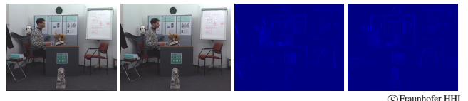
Figure 13: Ground truth comparison showing a known ground truth image (left) versus our warped image (middle left), and absolute difference images of warped and known ground truth for both baseline reduction (middle right) and extension (right).
