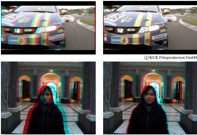
Figure 10: Automatic correction of disparity. The original stereo pairs are shown on the left, our result is on the right. The cropped racing car captured with strong negative disparities and a large overall scene depth results in the so-called framing problem. With a simple linear disparity scaling the car is pushed behind the screen without increasing the background disparity. In the bottom example, taken with a consumer 3D camera, the subject was moving towards the camera and finally exceeded the maximum disparity range. In our result, the global disparity range has been adapted so that the background remains at constant depth while the foreground is pushed closer to the screen.
