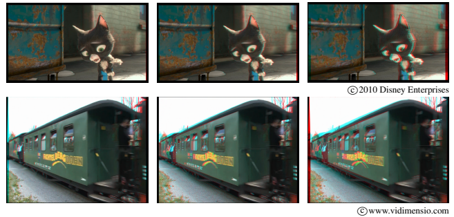
Figure 11: Display adaptation into both directions. The middle images are the original stereo pairs, while the left images feature a linear reduction of the disparity range to 50% and the right images an increase to 200%. These results show that our method allows to preserve the initial depth structure relative to the screen geometry to adapt content to actual viewing conditions.
