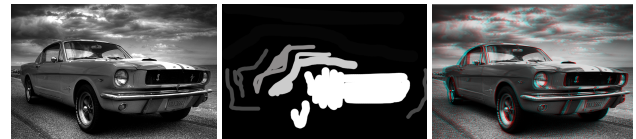
Figure 12: 2D to 3D conversion. From a single 2D input image and providing only a sparse set of disparity cues shown as rough scribbles, our method produces a convincing 3D result.
