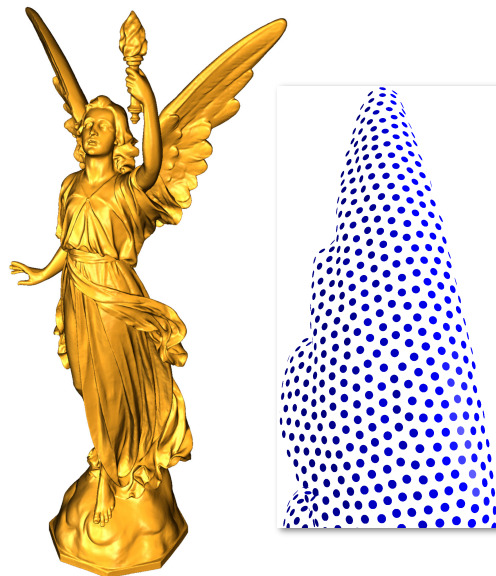
Figure 1: Left: The original model with 14 million samples is adaptively subsampled to 300k samples and reconstructed. Total time including out-of-core simplification and reconstruction is 6 minutes. Right: Detail from uniform resampling of the model to 21k samples.
