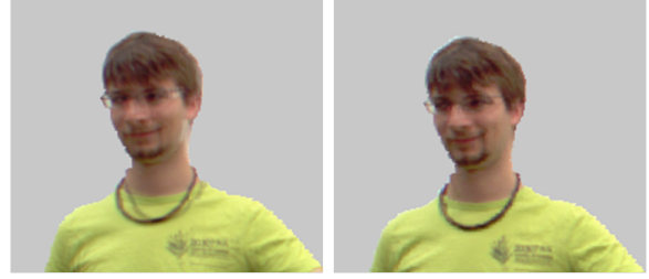
Figure 4: Photo-consistent blending. (Left) Basic rendering using angle-based weights, as in [BBM*01]. Note the ghosting of the necklace and general blurring. (Right) FreeCam photo-consistent blending.
