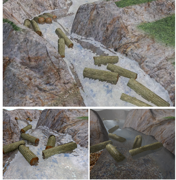
Figure 8: A dam built of several logs collapses, resulting in the fluid and the debris to flow down the valley. An unbounded domain is used, and the particles can flow to arbitrary locations. The bottom row shows different rendering techniques; on the left the surface is rendered offline with Povray, and on the right we used our real-time OpenGL renderer.
