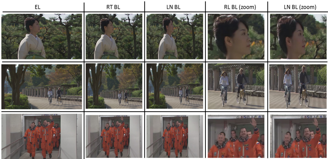
Fig. 4. Comparison between enhancement layers (EL) and base layers created by content-adaptive retargeting (RT BL) and linear scaling (LN BL) for the sequences Kimono1, ParkScene, and Crew. Note that EL has HD resolution while RT BL and LN BL have SD resolution.
