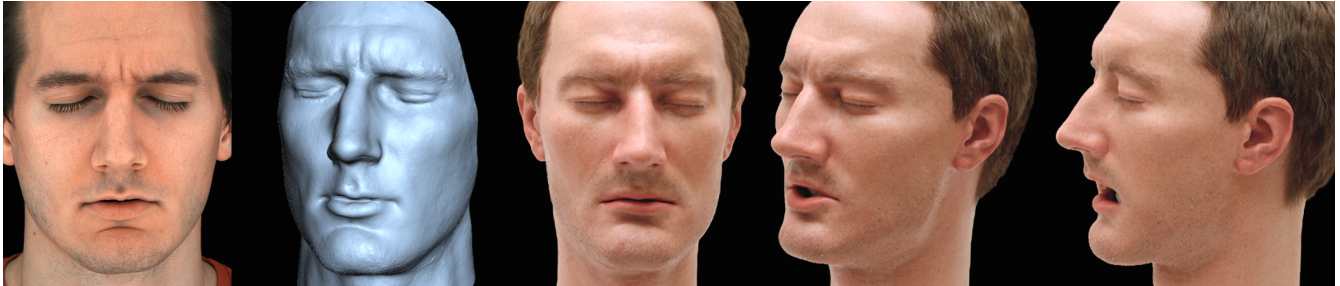
Figure 1: Left: photograph and scanned 3D geometry of a human face. We use a physics-based optimization process to design the geometry of a synthetic skin in order to best match given target expressions. Right: final animatronic figure with fabricated skin.
