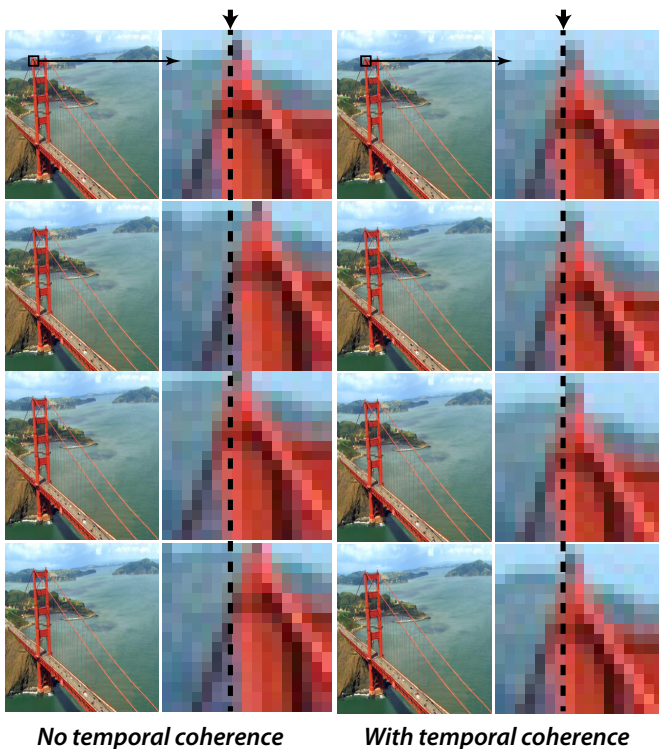
Fig. 18: Example of temporal stability of aspect ratio retargeting. Four consecutive frames of a video sequence with slow camera are shown, both without temporal coherence constraints and with temporal coherence constraints. To illustrate the effect of the coherence constraints better, we show a zoomed portion of the image with a vertical line as column reference. Without temporal constraints, the top of the bridge slightly moves left and right, which is perceived as a 'wobbling effect'. Using temporal constraints, such erroneous motion can be suppressed effectively. (Image sequence: ©Mammoth HD).
