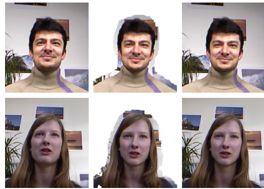
Figure 3: Left: original image from the color camera (i.e. without correct gaze). Middle: eye contact achieved by rotating the entire scene. Right: our method. Transferring the rotated face onto the original image does not lead to perspective aberrations.
