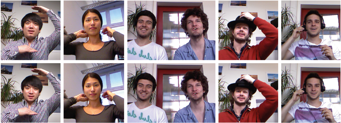
Figure 1: Top: frames recorded during video-conferencing. Note the lack of eye contact because of the disparity between the locations of the participant and the camera. Bottom: real-time gaze correction with the proposed algorithm.
