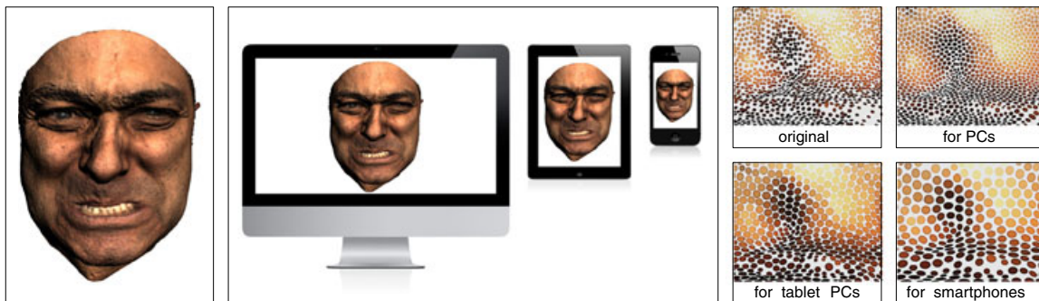
Figure 1. A facial model (left, 1201k points) is rendered by adaptive surface splatting in various devices. Adaptive surface splatting optimizes the facial model for PCs, tablet PCs, and smartphones. The middle figure is rendered according to the rendering performance and resolution of various devices, and the right figures show the splats, which are changed by desired density and a change of color and geometry on the surface.
