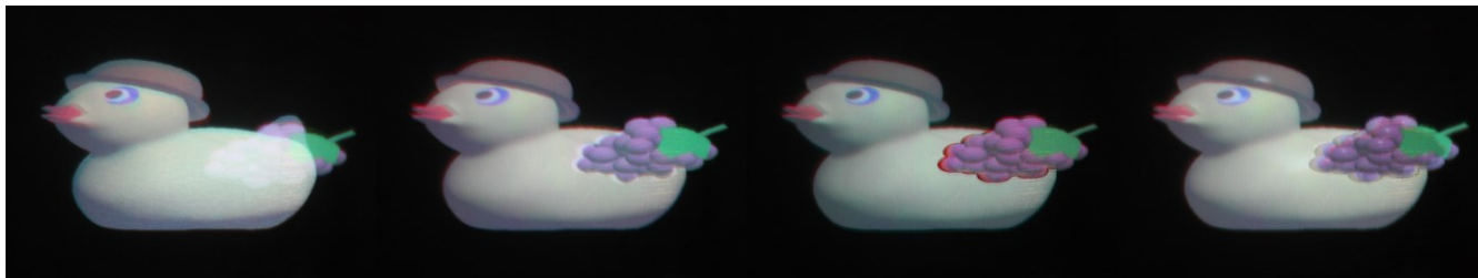
Figure 1: Illustration of the steps of our light field decomposition. (1) volumetric rendering, (2) view-independent and (3) view-dependent occlusion culling, (4) view-dependent rendering on parallax type layer. Photographs are taken from our multi-layered display prototype.
