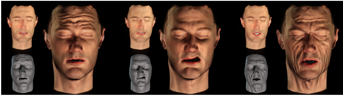
Figure 10: Three captured results of extreme poses, generated with our system. For every frame, the desired appearance is on the bottom left, and the robot configuration, under uniform white illumination, is on the top left.
