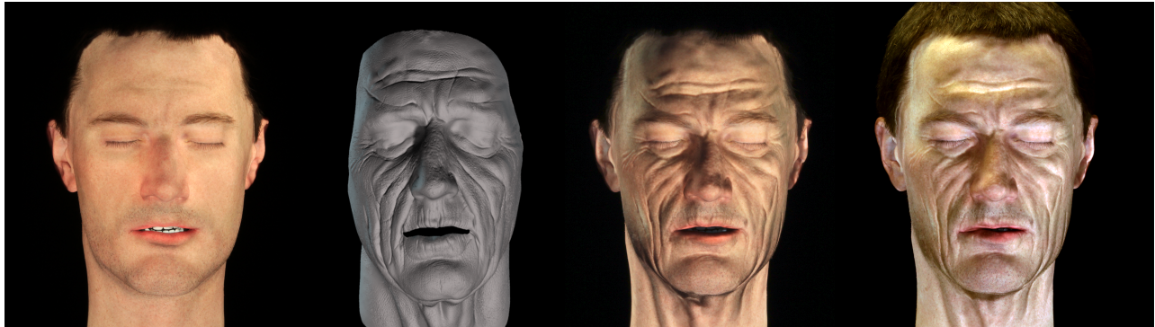
Figure 1: Our system allows augmentation of a physical avatar (left) with projector-based illumination, significantly increasing its expressiveness.
