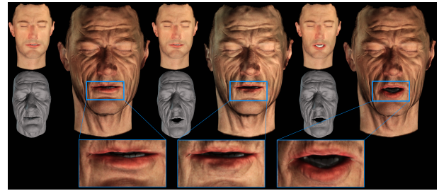
Figure 12: The neutral pose (left) of a sequence, compared to an extreme pose while the animatronic head is kept static (middle), and while it is actuated according to the proposed method (right). The head configuration under uniform illumination, and the target appearances are shown to the left of each result.
