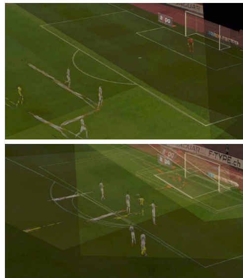
Fig. 3: Drift in long-term estimation due to error accumulation from frame-to-frame estimation. (30th (top) and 120th frames)
