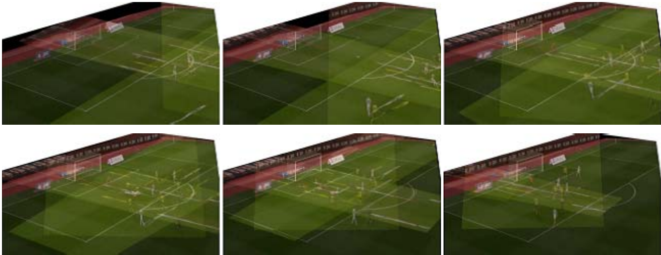
Fig. 6: Alignment of 3 cameras to master view for frames 0-271.
