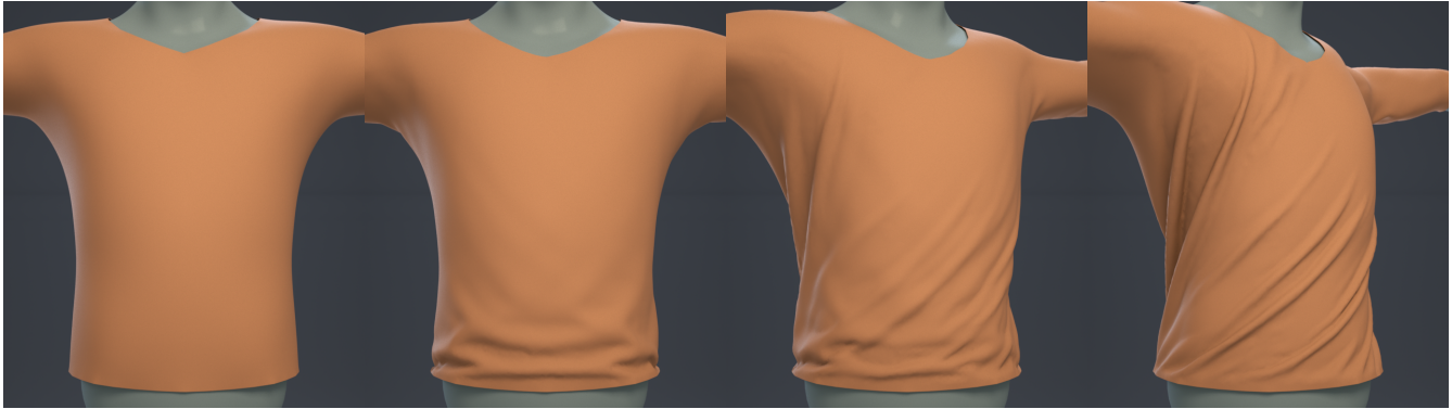
Figure 1: Example result of our method: A close-fitting sweater exhibits wrinkles and torsional folds under the effects of gravity and as the underlying torso is twisting. This example used only 12 adaptively chosen basis vectors and ran 18 times faster than a full simulation.
