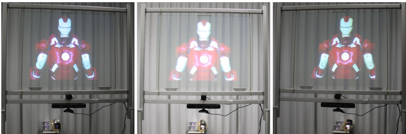
Figure 2: Results captured on our prototype. Three different viewing positions are shown in the three images. Left and right images are filtered with the corresponding linear polarizer to simulate the effect of polarized glasses in addition to the change of perspective. The center image was captured without any filter and thus both views are overlaid. The three images together illustrate image separation and crosstalk as well as motion parallax.
