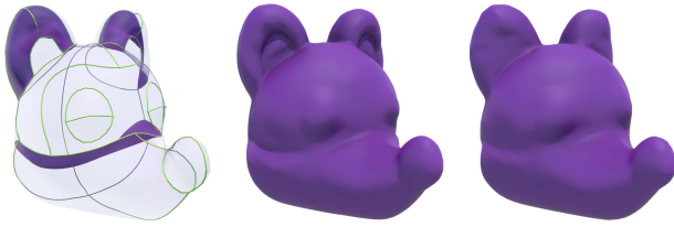
Figure 2: Internal connections (left) allow the designer to realize shapes with sharp creases and concave features (middle) that would be poorly approximated without internal structures (right).
