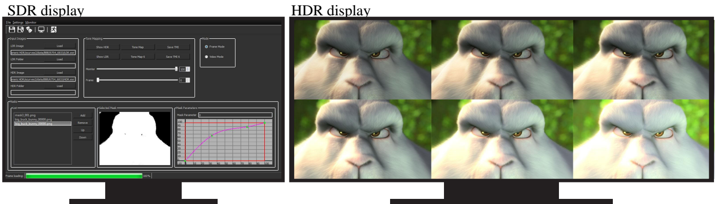
Figure 4: This figure shows our luminance grading interface. On the SDR display, masks with values in [0, 1] can be loaded in the bottom left menu, and are displayed in the bottom-middle window. A cubic spline interface shown on the bottom right allows the user to manually input lumipaths. Different visualization options can be selected from the menu on the top. On the HDR display, users can visualize their edits in an interactive manner. To see a standard work session using our interface, we point the reader to the supplementary material of this paper.
