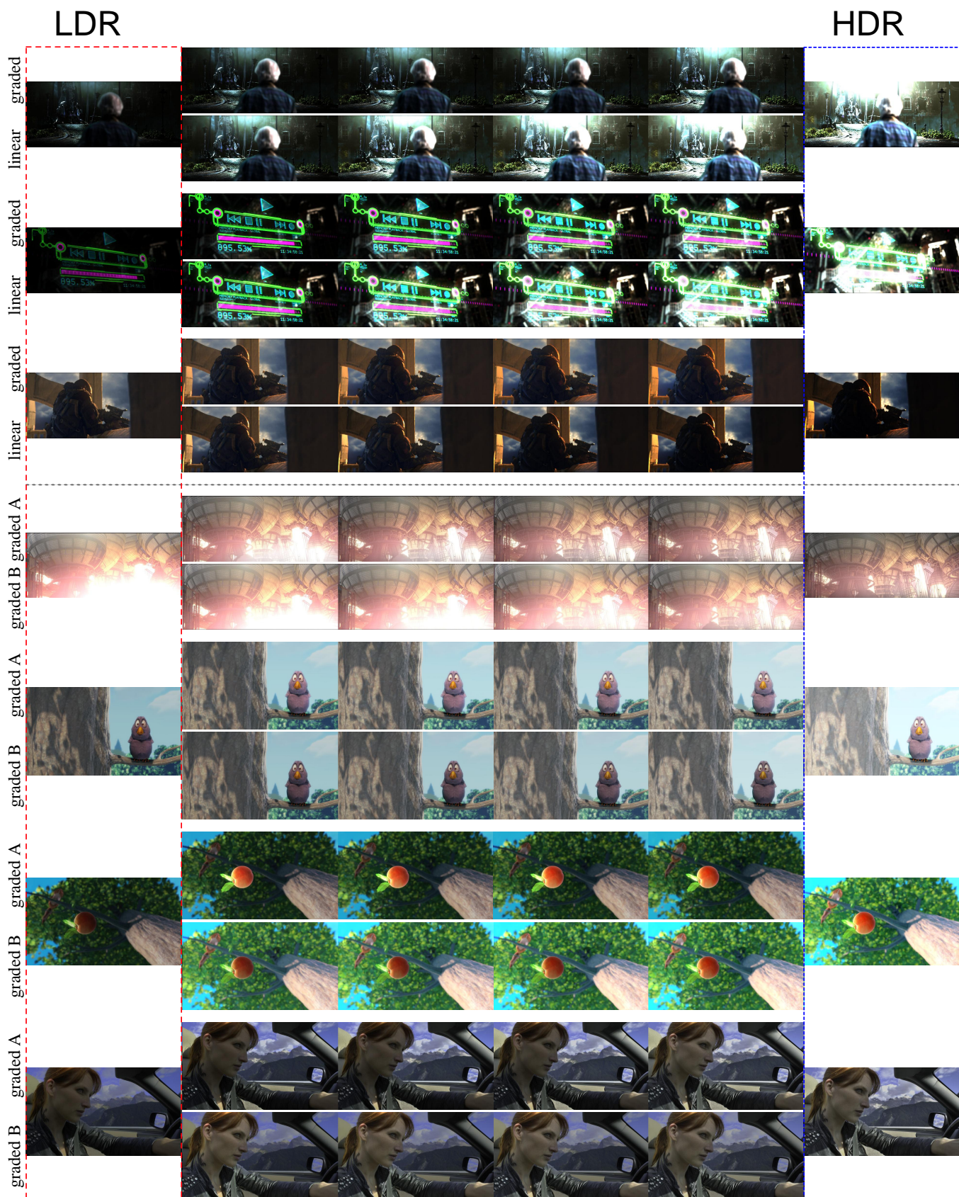
Figure 11: (Top) shows a comparison of results color graded with our method, as compared to a naive linear interpolation between the SDR and HDR graded versions. Notice that our system allows for local control of the grading at each point of the dynamic range hull. (Bottom) Two gradings obtained using our system are shown in contrast to showcase different artistic possibilities that can be achieved using our system.
