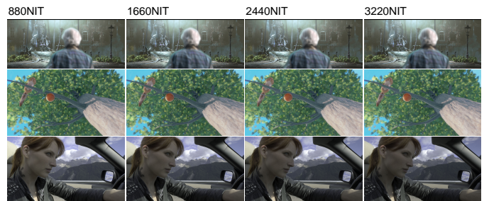
Figure 9: Display Adaptive Tone Mapping can be used to generate content for displays with different luminance levels, but does not allow for precise artistic control of content.
