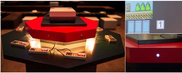
Figure 6: Game setup for the 360 degree projection configuration. Left: The console is set on a designated octagonal table in the middle of the room. Eight gamepads are connected to it in a circular manner. Top right: The active gamepad number is indicated next to the playing region at all times. Bottom right: an indicator light is illuminated when the corresponding gamepad is active.
