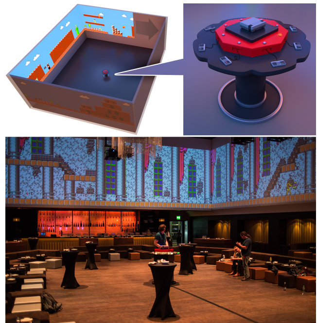
Figure 1: Side-scrolling games unfold across the walls of the room to encircle the players, immersing them into the game's world. The games are played using the console, enhanced to allow up to eight players to participate, in the center of the room.
