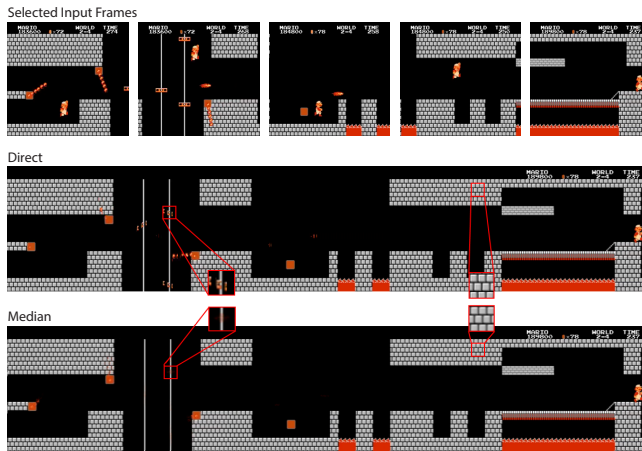
Figure 4: Comparison of frame composition modes. The direct mode does not suppress foreground elements and can result in artifacts that include stretching, squeezing, and tearing of foreground objects. The median mode suppresses foreground objects but can sometimes lead to blurring. Examples are highlighted by enlarged patches.
