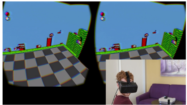
Figure 5: VR setup. Employing the Oculus Rift DK2, the tracked buffer spans across four walls in a scene inspired by the 360 degree projection setup. In the main image, the views shown to the player's eyes are presented. The player, shown in the lower right, enjoys a life-sized game realm as it unfolds during gameplay.
