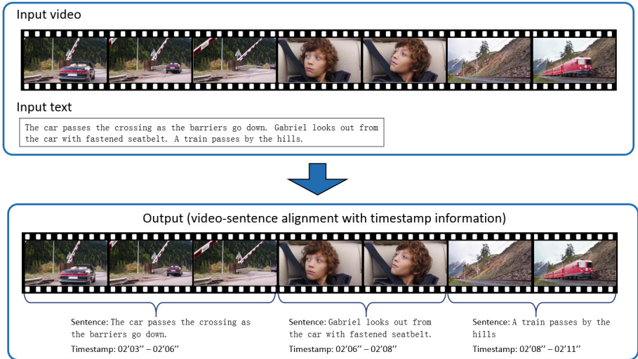
Fig. 1. Given an input movie and associated narrative sentences (e.g. from the movie script), our approach temporally aligns the video frames with the sentences and provides the timestamp information of the sentences. This figure illustrates a representative result for a 10-minutes long continuous video from the movie Lucid Dreams of Gabriel . For a better visibility of the figure, only a 8-seconds segment is shown here.
