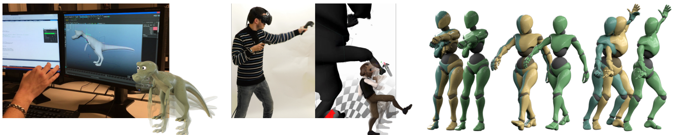
Figure 9: Our system supports a variety of performance capture devices. Here we show a jump cycle created using the Leap Motion hand tracker (left), a kick cycle created using the HTC Vive (middle), and a punch, a walk and a samba cycles created using a full body motion-capture suit (right). In these last examples, the overlapped blue and yellow mannequins show the spatial difference of cycles in the imperfect performed motion, while the green mannequin shows the looping cycle extracted by our algorithm. Note that in each case, we solve for a single multidimensional curve representing the whole motion (dimension 127 for the punch cycle, 254 for the walk cycle and 160 for the samba cycle).
