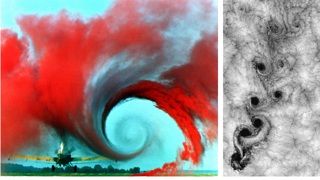
Figure 1: Examples of real-world air flows. Left: wake vortex study of an agricultural plane (image from the NASA Langley Research Center), right: clouds off the Chilean coast near the Juan Fernandez Islands form a von-Kármán vortex street (by Bob Cahalan, NASA Goddard Space Flight Center). Both images are in public domain.
