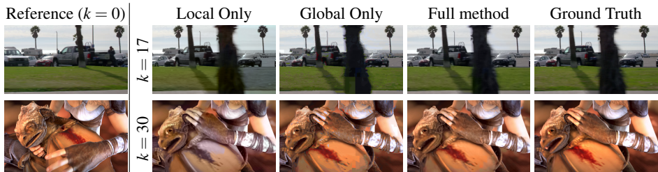
Figure 4: Ablation study. Using local color propagation based on [53] only preserve details but is sensitive to occlusion/dis-occlusion. Using only global color transfer does not preserve details and is not temporally stable. Best result is obtained when combining both strategies. See Figure 9 for quantitative evaluation. (Image source: [0, 47])
