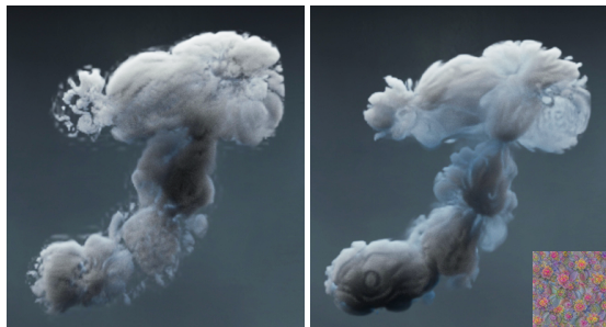
Fig. 5. Value-based (left) against transport-based density optimization (right) with a flower motif 0 . The value-based approach used in traditional image stylization approaches produces ghosting artifacts and thinner smoke structures, since density sources can be created and removed to match targeted features.
