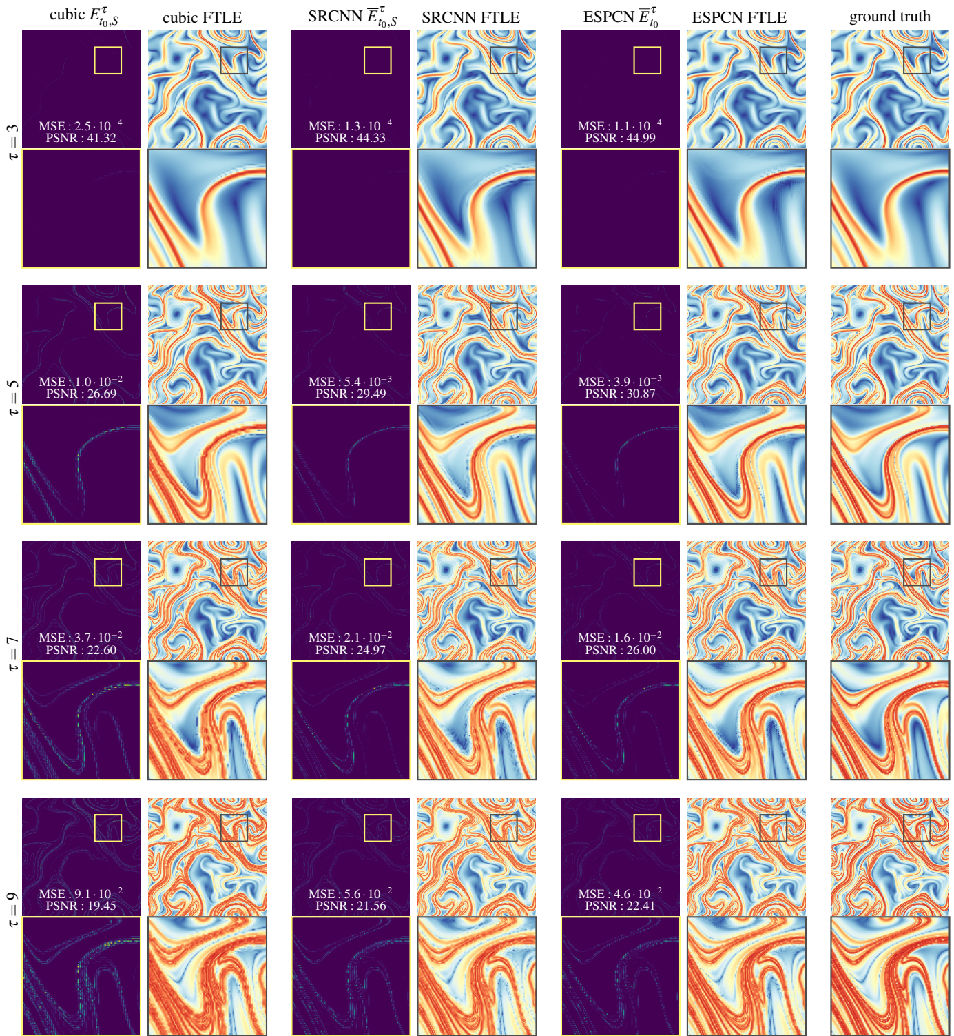
Fig. 1: Error maps and FTLE comparisons in our simulated flow #2000 for different integration durations \tau . Here, for a 2\times upsampling.
