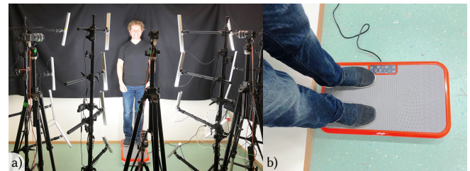
Fig. 2. Capture Setup: We use a multi-view capture setup for reconstructing facial performances (a). In addition to capturing motions such as walking or jumping, we also employ a vibrating "step" platform that oscillates at varying speeds in order to induce controllable and repeatable dynamic effects (b).
