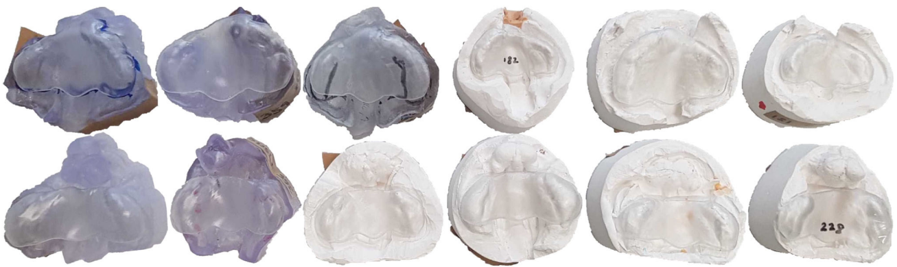
Fig. 4 Automatically computed and 3D-printed plates given twelve different intraoral scans and plaster cast impressions—top UCLP, bottom BCLP. Two cleft care professionals assessed each plate's suitability based on its shape and its fit on the corresponding palate model
